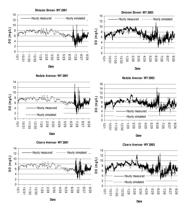
**Figure 3.35** Comparison of measured and simulated dissolved oxygen (DO) concentrations at Division Street, Kedzie Avenue, and Cicero Avenue on the Calumet-Sag Channel for Water Years 2001 and 2003
