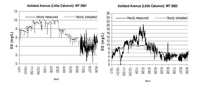
**Figure 3.40** Comparison of measured and simulated dissolved oxygen (DO) concentrations at Ashland Avenue on the Little Calumet River (South) for Water Years 2001 and 2003
