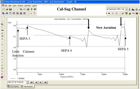
**Figure 4.22** Dissolved oxygen concentration profiles in the Chicago Waterway System for selected critical periods of July 24, 2001 (Little Calumet River north) and July 26, 2001 (Cal-Sag Channel) where the downward arrows indicate locations of new aeration stations
