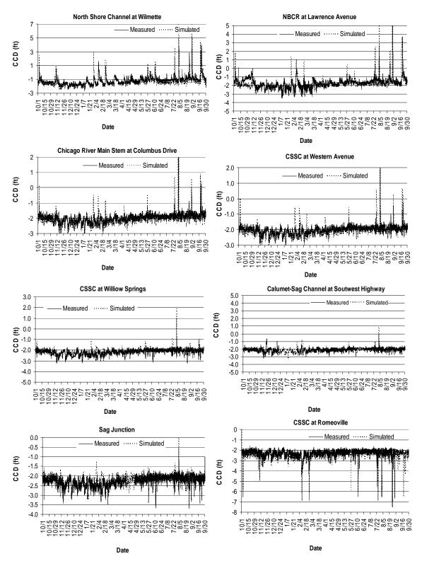
**Figure 2.6** Measured and simulated water-surface elevations relative to the City of Chicago Datum (CCD) at different locations in the Chicago Waterway System for October 1, 2000 to September 30, 2001 (Water Year 2001)
