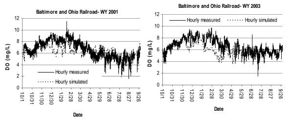
**Figure 3.30** Comparison of measured and simulated dissolved oxygen (DO) concentrations at the Baltimore and Ohio Railroad on the Chicago Sanitary Ship Canal for Water Years 2001 and 2003
