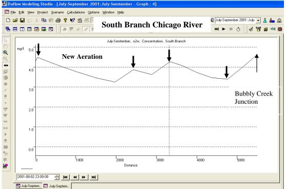
**Figure 4.20** Dissolved oxygen concentration profiles in the Chicago Waterway System for selected critical periods of August 4, 2001 (Chicago River Main Stem) and August 2, 2001 (South Branch Chicago River) where the downward arrows indicate locations of new aeration stations
