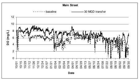
**Figure 4.10** Simulated hourly DO concentrations at Linden Street, Simpson Street, and Main Street on the NSC for a 30 MGD transfer of aerated effluent from the NSWRP to the upstream end of the NSC compared with baseline simulated concentrations for WY 2001
