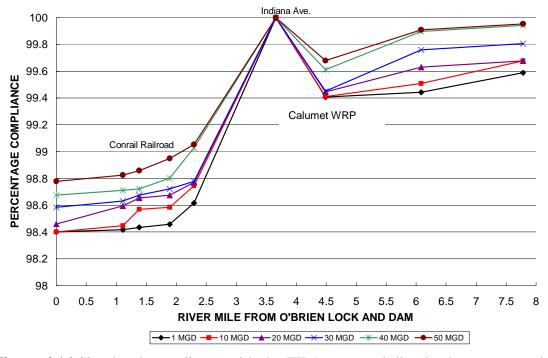
**Figure 4.16** Simulated compliance with the IEPA proposed dissolved oxygen standards for Water Year 2001 upstream from O'Brien Lock and Dam to Division Street on the Calumet-Sag Channel (0.6 mi upstream from SEPA station 3) for different amounts (in million gallons per day, MGD) of aerated flow transfer.
