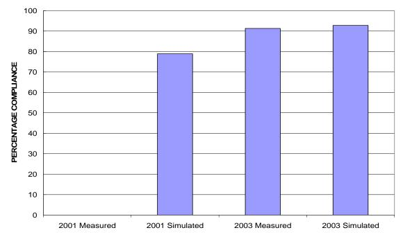
**Figure 4.6** Measured and simulated compliance with the IEPA proposed dissolved oxygen (DO) standards on Bubbly Creek at Interstate 55. (note: no measured DO data were available for WY 2001 at this location)
