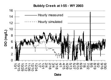
**Figure 3.42** Comparison of measured and simulated dissolved oxygen (DO) concentrations at I-55 on Bubbly Creek for Water Year 2003
