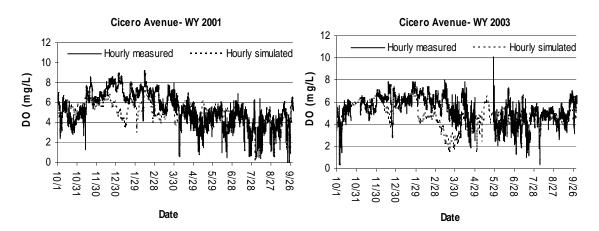
**Figure 3.29** Comparison of measured and simulated dissolved oxygen (DO) concentrations at Cicero Avenue on the Chicago Sanitary and Ship Canal for Water Years 2001 and 2003
