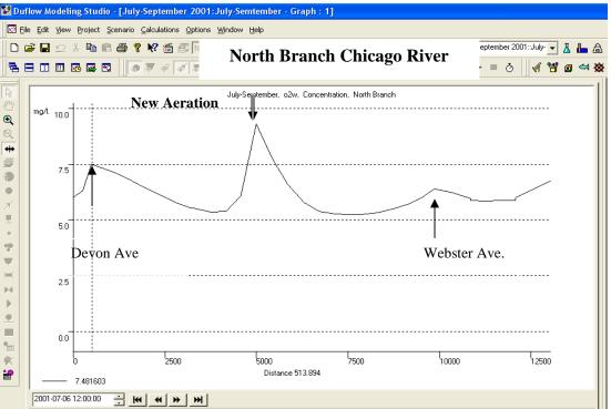
**Figure 4.19** Dissolved oxygen concentration profiles in the Chicago Waterway System for selected critical periods of August 2, 2001 (North Shore Channel) and July 6, 2001(North Branch Chicago River) where the downward arrows indicate locations of new aeration stations
