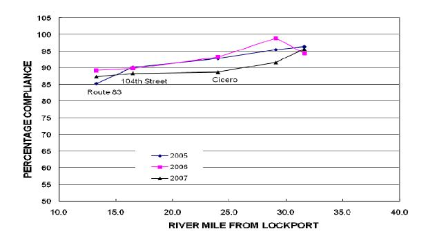
**Figure 4.8** Measured percentage compliance with the IEPA proposed dissolved oxygen standards for calendar years 2005-2007 along the Little Calumet River (North) and Calumet-Sag Channel.
