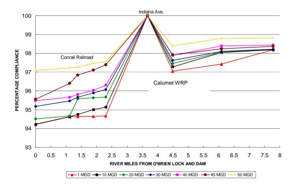
**Figure 4.17** Simulated compliance with the IEPA proposed dissolved oxygen standards for Water Year 2003 upstream from O'Brien Lock and Dam to Division Street on the Calumet-Sag Channel (0.6 mi upstream from SEPA station 3) for different amounts (in million gallons per day, MGD) of aerated flow transfer.
