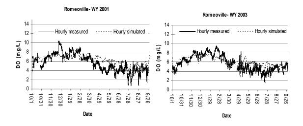
**Figure 3.33** Comparison of measured and simulated dissolved oxygen (DO) concentrations at Romeoville on the Chicago Sanitary and Ship Canal for Water Years 2001 and 2003
