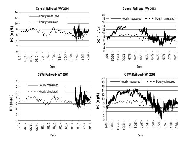
**Figure 3.41** Comparison of measured and simulated dissolved oxygen (DO) concentrations at Conrail Railroad and the Central and Wisconsin Railroad on the Little Calumet River (North) for Water Years 2001 and 2003
