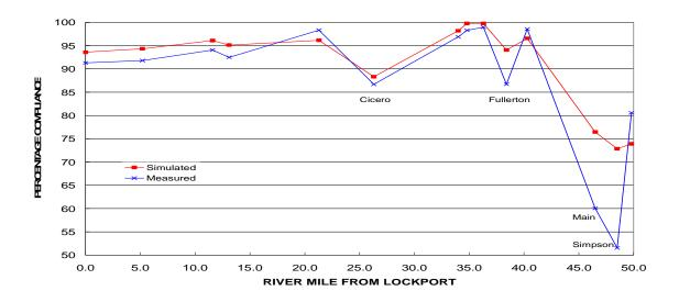
**Figure 4.2** Simulated and measured compliance with the IEPA proposed dissolved oxygen standards for Water Year 2001 along the North Shore Channel, North Branch, South Branch, and Chicago Sanitary and Ship Canal.
