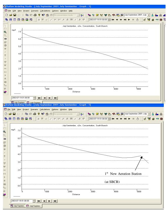
**Figure 5.6** Identification of the new aeration station new aeration station locations on the South Branch Chicago River (SBCR) for WY 2003, where the upper and lower figures show the DO concentration along the SBCR without and with supplemental aeration, respectively, for 1 a.m. on July 19, 2003
