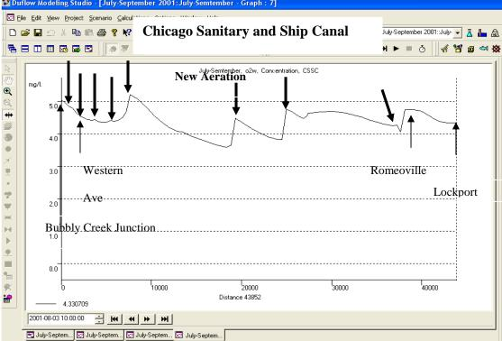
**Figure 4.21** Dissolved oxygen concentration profiles in the Chicago Waterway System for a selected critical period of August 3, 2001 (Bubbly Creek and Chicago Sanitary and Ship Canal) where the downward arrows indicate locations of new aeration stations
