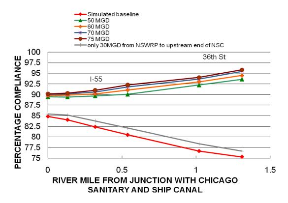
**Figure 4.13** Simulated compliance with the IEPA proposed dissolved oxygen standards for Water Year 2001 along Bubbly Creek for different amounts (in million gallons per day, MGD) of unaerated flow transfer.
