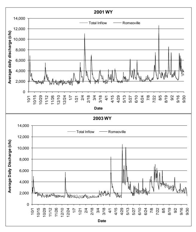
**Figure 2.5** Comparison of the summation of all measured or estimated (except gravity combined sewer overflows) inflows (Total) and the measured outflow at Romeoville for October 1, 2000 to September 30, 2001 (Water Year 2001) and October 1, 2002 to September 30, 2003 (Water Year 2003)
