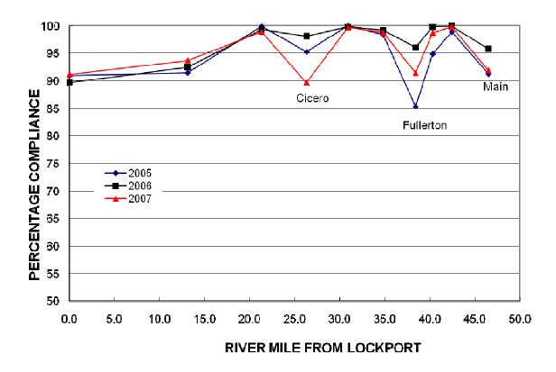
**Figure 4.7** Measured percentage compliance with the IEPA proposed dissolved oxygen standards for calendar years 2005-2007 along the North Shore Channel, North Branch, South Branch, and Chicago Sanitary and Ship Canal.
