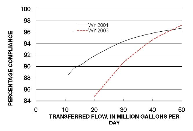
**Figure 4.9** Percentage compliance with the IEPA proposed dissolved oxygen standards at Main Street on the Upper North Shore Channel (UNSC) as a function of the transfer of aerated effluent from the North Side Water Reclamation Plant to the upstream end of the UNSC.
