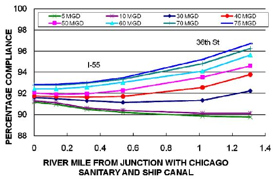
**Figure 4.11** Simulated compliance with the IEPA proposed dissolved oxygen standards for Water Year 2001 along Bubbly Creek for different amounts (in million gallons per day, MGD) of aerated flow transfer.
