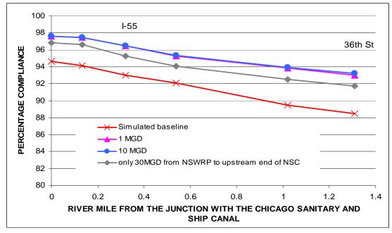
**Figure 4.14** Simulated compliance with the IEPA proposed dissolved oxygen standards for Water Year 2003 along Bubbly Creek for different amounts (in million gallons per day, MGD) of unaerated flow transfer.
