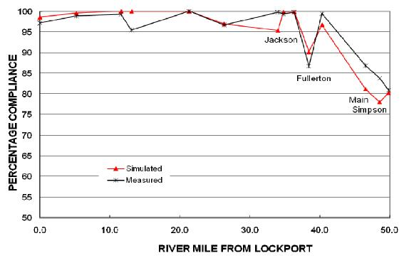
**Figure 4.3** Simulated and measured compliance with the IEPA proposed dissolved oxygen standards for Water Year 2003 along the North Shore Channel, North Branch, South Branch, and Chicago Sanitary and Ship Canal.
