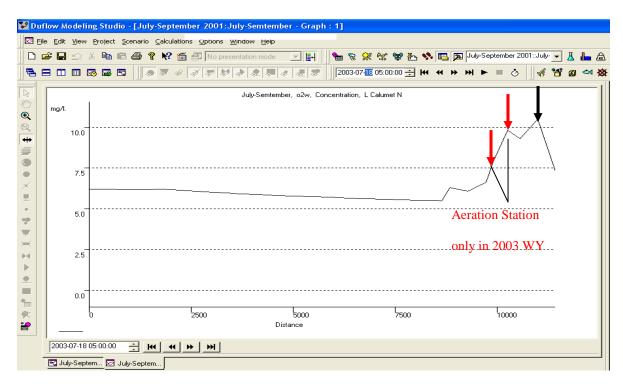
**Figure 4.23** Dissolved oxygen concentration profiles in the Chicago Waterway System for selected critical periods of October 1, 2003 (North Branch Chicago River) and July 18, 2003 (Little Calumet River North) where the downward arrows indicate locations of new aeration stations
