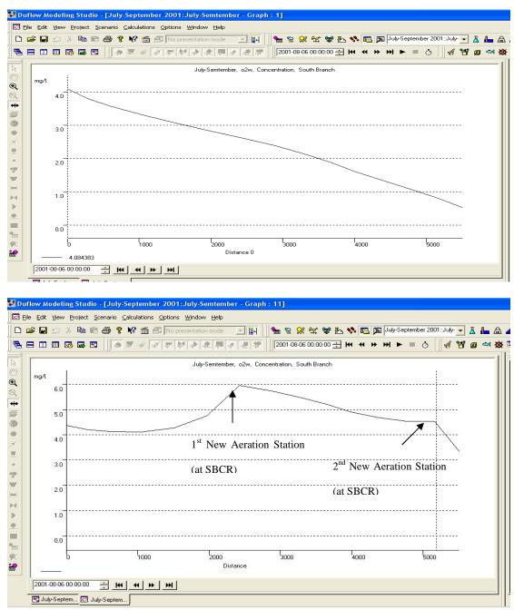
**Figure 5.3** Identification of new aeration station locations on the South Branch Chicago River (SBCR) for WY 2001, where the upper and lower figures show the dissolved oxygen concentration along the SBCR without and with supplemental aeration, respectively, for midnight on August 6, 2001
