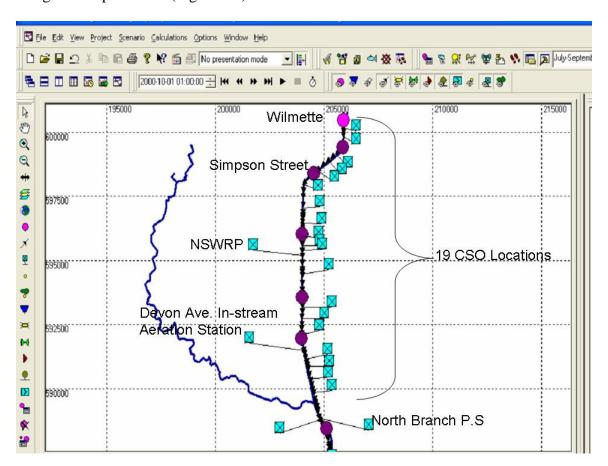
**Figure 2.1** Location of the 19 representative gravity CSOs on the North Shore Channel in the improved DUFLOW model
