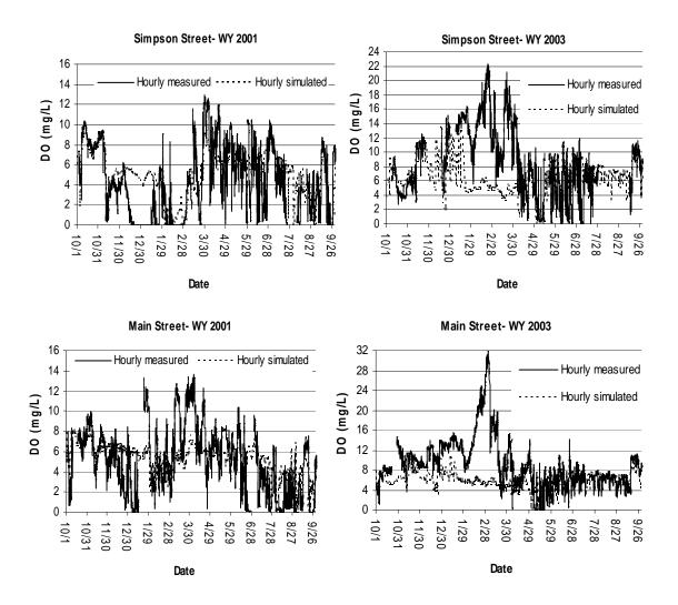
**Figure 3.38** Comparison of measured and simulated dissolved oxygen (DO) concentrations at Simpson and Main Streets on the North Shore Channel for Water Years 2001 and 2003
