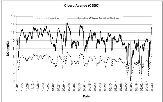
**Figure 5.2** Dissolved Oxygen (DO) concentrations for the baseline and integrated strategy simulations on the South Branch Chicago River and Chicago Sanitary and Ship Canal for Water Year 2001
