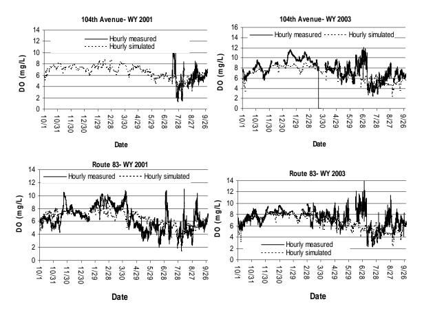
**Figure 3.37** Comparison of measured and simulated dissolved oxygen (DO) concentrations at 104<sup>th</sup> Avenue and Route 83 on the Calumet-Sag Channel for Water Years 2001 and 2003
