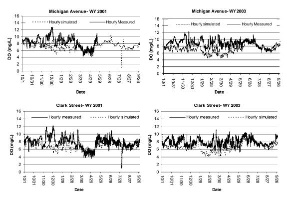
**Figure 3.39** Comparison of measured and simulated dissolved oxygen (DO) concentrations on the Chicago River Main Stem at Clark Street and Michigan Avenue for Water Years 2001 and 2003
