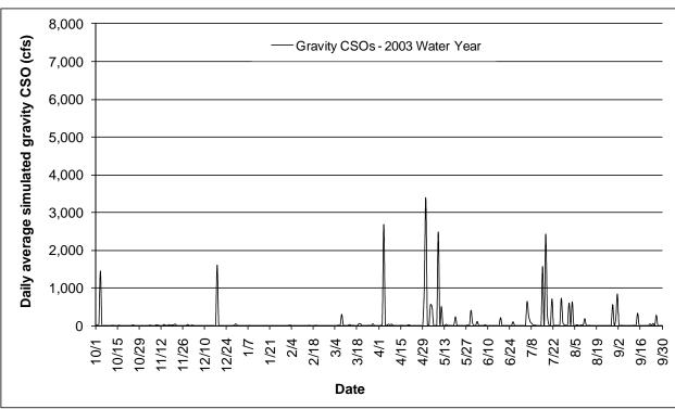
**Figure 2.4** Daily average simulated gravity combined sewer overflow (CSO) flows obtained from the U.S. Army Corps of Engineers
