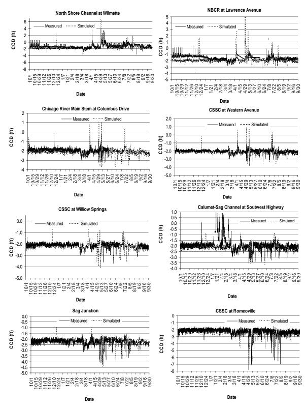
**Figure 2.7** Measured and simulated water-surface elevations relative to the City of Chicago Datum (CCD) at different locations in the Chicago Waterway System for October 1, 2002 to September 30, 2003 (Water Year 2003)
