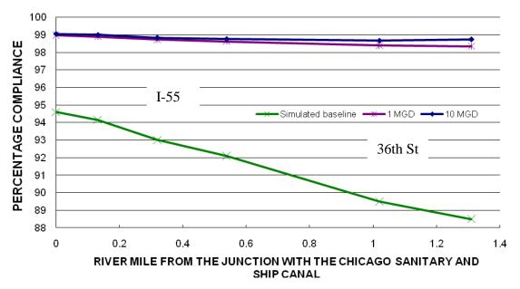
**Figure 4.12** Simulated compliance with the IEPA proposed dissolved oxygen standards for Water Year 2003 along Bubbly Creek for different amounts (in million gallons per day, MGD) of aerated flow transfer.
